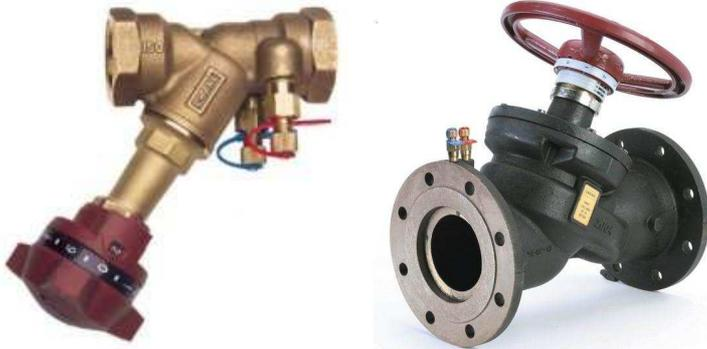
This combined assembly traditionally was assembled from a double regulating valve and fixed orifice device. More commonly nowadays the orifice is fitted directly into the body of the valve.
