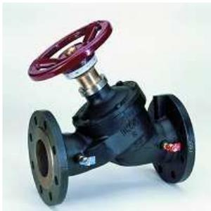
This indicates that the differential pressure will be measured across the entire valve. If this is the case then the size of the orifice will change when the valve is operated. This valve is therefore a **Variable Orifice Double regulating valve (VODRV)**
