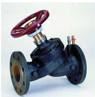
If the valve is fitted with testpoints that are very close together when measured along the axis of the pipe then the valve is likely to be a **Fixed Orifice Double Regulating Valve (FODRV)**
