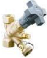
The Oventrop example here shows a combined testpoint and drain unit very close to another testpoint. This valve is a variable valve. The testpoint nearest to the centre of the valve is ported downstream of the valve seat.
