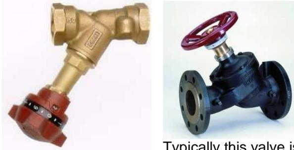
Typically this valve is a Y pattern globe valve arranged in this way to present the smallest pressure loss to the system when fully open. Adjustment of this valve will add resistance to the system and hence reduce the flow. The description DOUBLE regulating means that it has a feature whereby you can set the position that the valve is to operate at in such a way that you can still close the valve for maintenance purposes.
