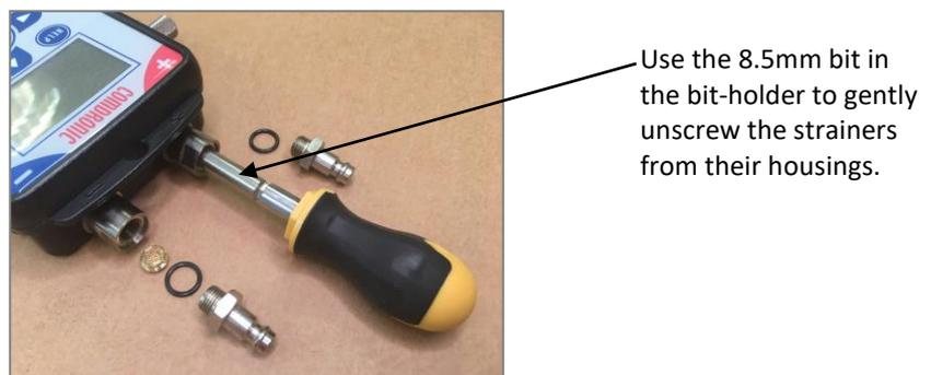
Step 3 – If the strainers are being reused, clean them in a soapy solution and then flush them with a pressurised air / water source.
