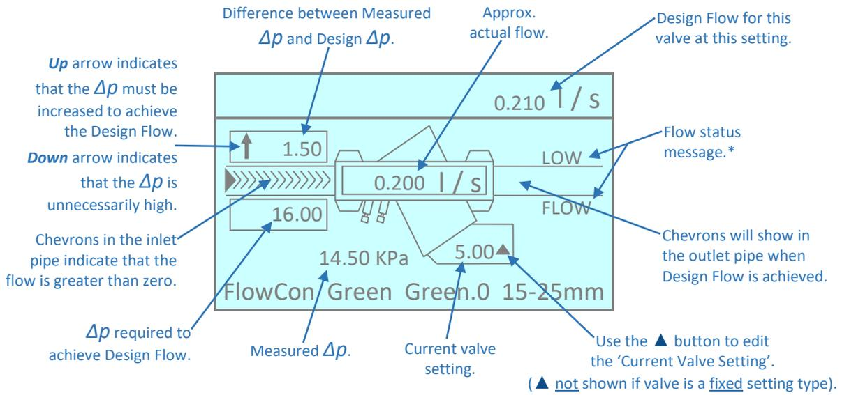
\*The Design Flow for any automatic balancing valve will be achieved if the  $\Delta p$  across the valve reaches (or exceeds) the design value. If the Design  $\Delta p$  is met, the displayed message will be **FLOW OK**. If the Design  $\Delta p$  is not met, the displayed message will be **LOW FLOW**.
