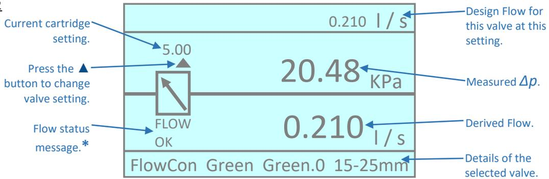
\*If the measured  $\Delta p$  reaches the design  $\Delta p$  for the selected valve, the flow status message will be **FLOW OK**. However, if the design  $\Delta p$  is not met the flow status message will be **LOW FLOW**.
