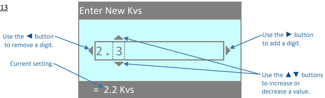
Once the new value is correct on the screen, press **OK** to accept it. Or, press **EXIT** to exit the screen and retain the current setting.
