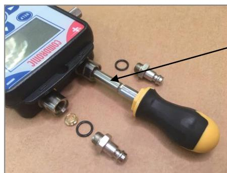
Use the 8.5mm bit in the bit-holder to gently unscrew the strainers from their housings.
