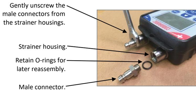
**IMPORTANT** - Take care not to disturb (i.e. move) the strainer housings. If a male connector doesn't readily unscrew, use a 14mm wrench to hold the strainer housing in place before any additional force is applied.
