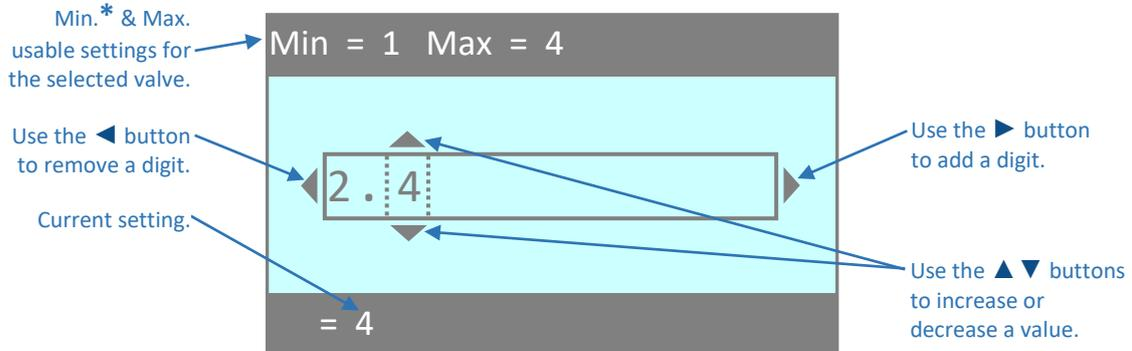
Once the new value is correct on the screen, press **OK** to accept it. Or, press **EXIT** to exit the screen and retain the current setting.
