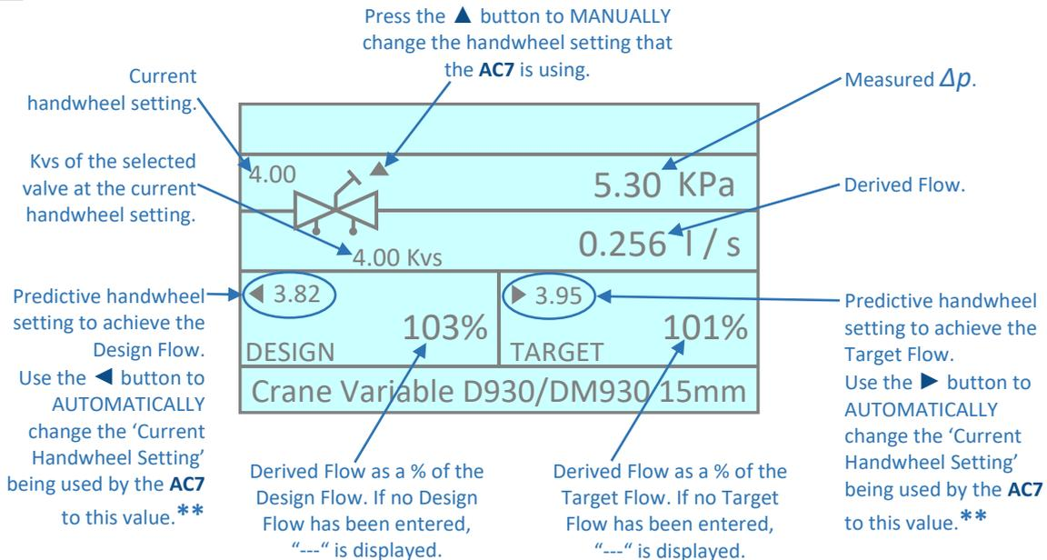
\*\*These are iterative processes due to the unknown valve authority in the circuit and so 2-3 attempts may be required to achieve the desired reading. Please also note that in conjunction with pressing the ◀ or ▶ button on the AC7, the physical handwheel setting of the valve will also need to be changed to match the new value.
