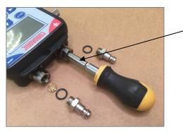
Use the 8.5mm bit in the bit-holder to gently unscrew the strainers from their housings.
