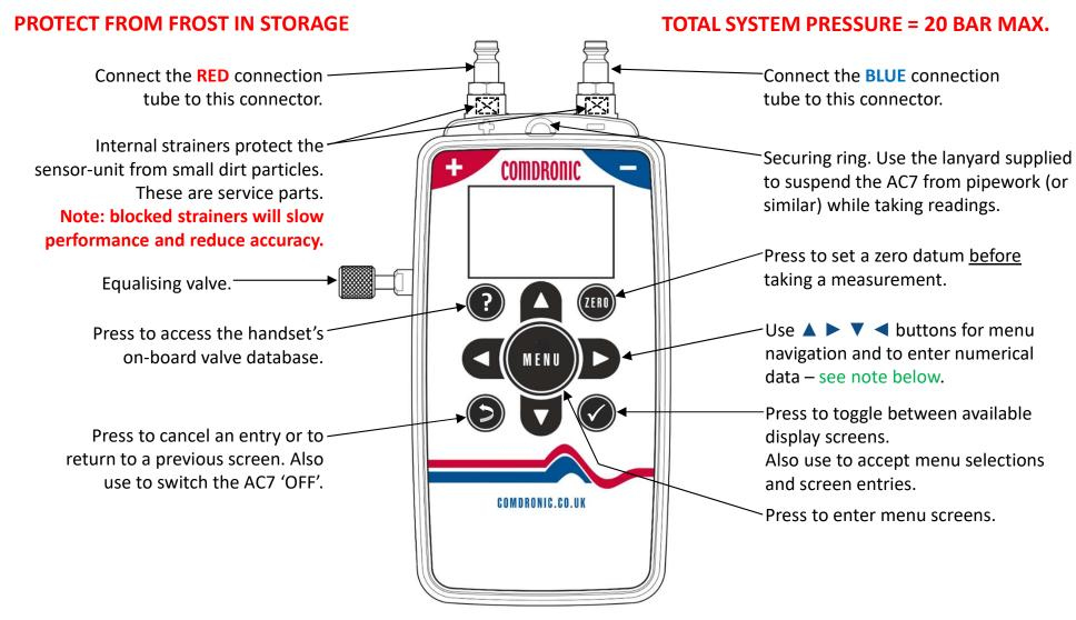
Numeric entries: use the ▲ ▼ buttons to increase or decrease values. Use the ▶ button to add a digit. If a decimal point is required, press the ▼ button when the zero digit is showing. To enter a negative number, press the ZERO button before any number is added.
