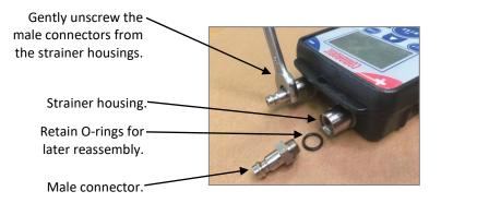
IMPORTANT - Take care not to disturb (i.e. move) the strainer housings. If a male connector doesn't readily unscrew, use a 14mm wrench to hold the strainer housing in place before any additional force is applied.
