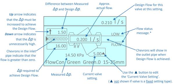
\*The Design Flow for any automatic balancing valve will be achieved if the  $\Delta p$  across the valve reaches (or exceeds) the design value. If the Design  $\Delta p$  is met, the displayed message will be **FLOW OK**. If the Design  $\Delta p$  is not met, the displayed message will be **LOW FLOW**.
