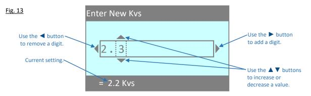
Once the new value is correct on the screen, press **OK** to accept it. Or, press **EXIT** to exit the screen and <u>retain</u> the current setting.
