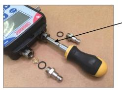
Use the 8.5mm bit in the bit-holder to gently unscrew the strainers from their housings.
