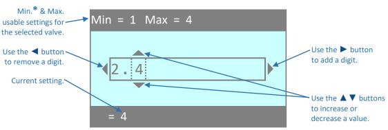
Once the new value is correct on the screen, press **OK** to accept it. Or, press **EXIT** to exit the screen and <u>retain</u> the current setting.
