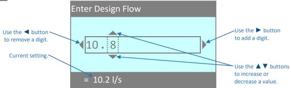
Once the new value is correct on the screen, press **OK** to accept it. Or, press **EXIT** to exit the screen and <u>retain</u> the current setting.
