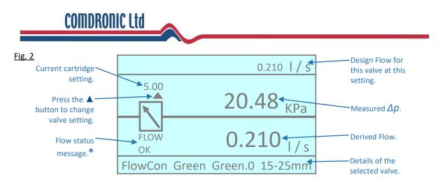
\*If the measured  $\Delta p$  reaches the design  $\Delta p$  for the selected value, the flow status message will be **FLOW OK**. However, if the design  $\Delta p$  is not met the flow status message will be **LOW FLOW**.
